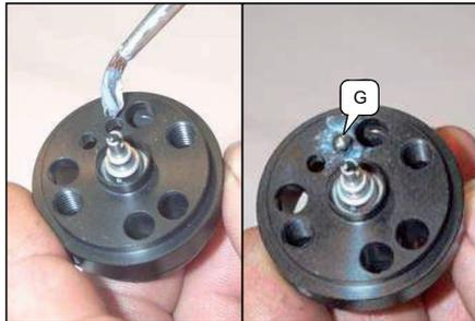
Apply o-ring lube to outside of housing adapter C and assemble to reverse housing assembly F while maintaining proper alignment of ball G and spring.
