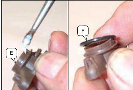
Lubricate the ID step on reverse block A with o-ring lube and assemble reverse valve E in place.
