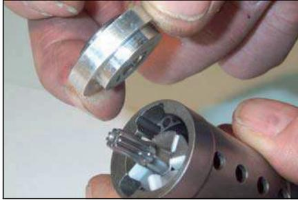
Place OM81-01 on top of motor, then press until bearing C is flush with the endplate B.
