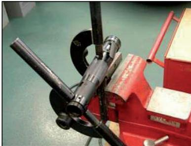
Make sure clutch assembly L is well lubricated, then slide it into housing, seat it on the 1st stage gearhead, and rotate to ensure free movement.
