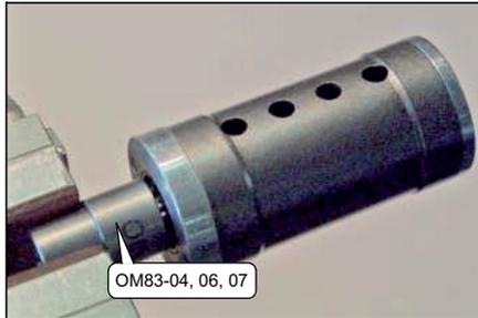
Heat the screw I in the rear of the motor with a heat gun.
