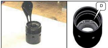
Slide spacer C on spindle assembly A. Place spindle assembly into gearcase F, check to ensure teeth match, and press assembly into bearing. Note: be sure to support bearing by inner race during press.
