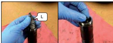
Take the clutch bearing, bearing cap, and spacer from 2nd stage module and place them on top of the clutch. By hand, lightly press on bearing cap until clutch is fully seated. Cap should be flush against the clutch housing and clutch should have less than 0.2mm of axial play (if more, add P/N 131908 to other side of clutch).
