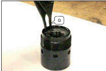
Place gearhead assembly D into gearcase E, check to ensure teeth match, and press assembly into bearing.
