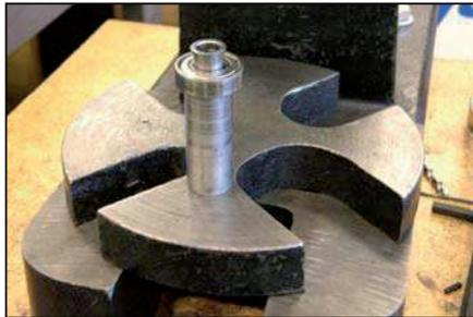
Slide pinion/bearing A/B into gearcase MAKING SURE gears are still aligned correctly.
