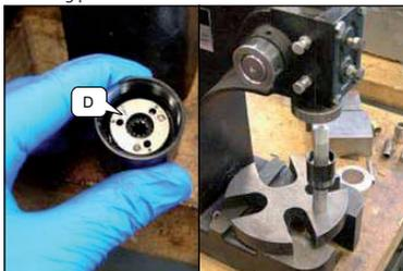
Check to ensure gearhead assembly D is fully pressed onto bearing (assembly will be below the top of the ring gear teeth).
