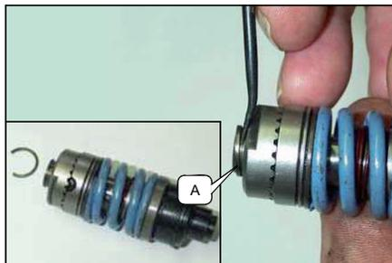
Remove adjustment nut B by rotating screw driver clockwise.
