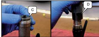
Rotate the output of the gearhead assembly by hand to ensure free movement.
