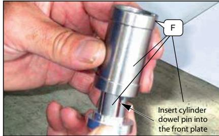
Place OM81-01/02 in the manual arbor press. Put the rear plate G on cylinder F. (Note: Pin in cylinder must be lined up with hole in endplate.) Install bearing H onto the rotor using the press and OM81-01/02. Press until entire assembly is tight and will not rotate.
