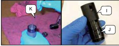
Screw clutch housing J onto motor housing.
