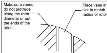
Mount the rotor & end plate assembly in the cylinder.
