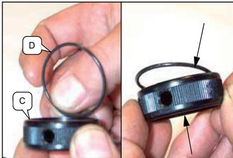
Coat the o-ring D with o-ring lube.
