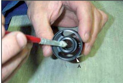
Using OM127, place valve seat B into housing A.
