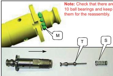
Clean the pieces of the clutch assembly using degreaser.
