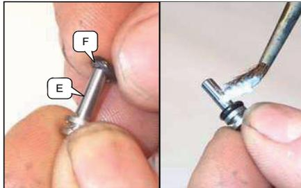
Install the valve E in the housing A using needle-nose pliers.
