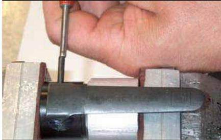
Place o-ring F over valve E and coat with o-ring lube.
