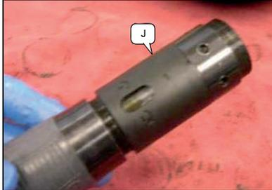
FOR ANGLE TOOLS: Tighten to 70 N-m using two spanner wrenches.
