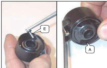
Coat the o-ring G with o-ring lube. Place o-ring G on the housing A.
