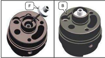
Assemble Dallas Chip C into hole on housing adapter B.
