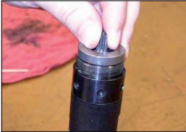
If bearing cap is not flush, use a shim gauge to measure the gap between the cap and the top of the clutch housing. Remove the quantity of layers of the spacer required to exceed measured gap. Note: axial play of clutch should be greater than 0.05mm but less than 0.20mm.
