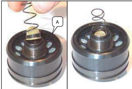
Compress and hold the exhaust assembly to the lever assembly.
