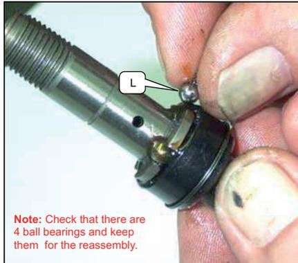
Remove the 6x2.38mm ball bearings M by and save them for reassembly.
