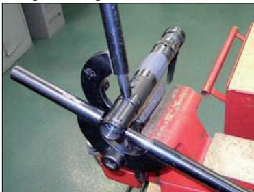
For the 055 angle tool, thread third stage on and use spanner wrenches to tighten to 70 N-m. For the 046 inline tool, tighten it to 40 N-m.
