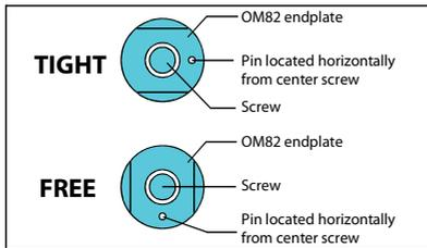
**Note:** When spacing is correct and motor is rotating freely, motor and OM82 should fall to vertical orientation of pin and center screw. If motor does not come free and screw cannot be tightened further, motor must be completely disassembled
