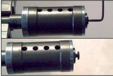
Lightly tap on rotor spline with plastic mallet to push rotor D out of endplate B. Remove motor parts one at a time.
