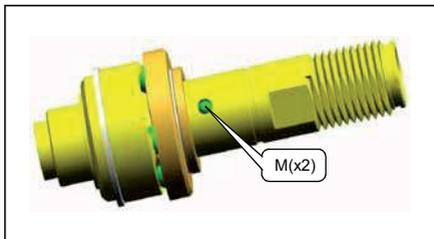
Assemble the shutoff collar J, the spring I, and the clutch guide H.
