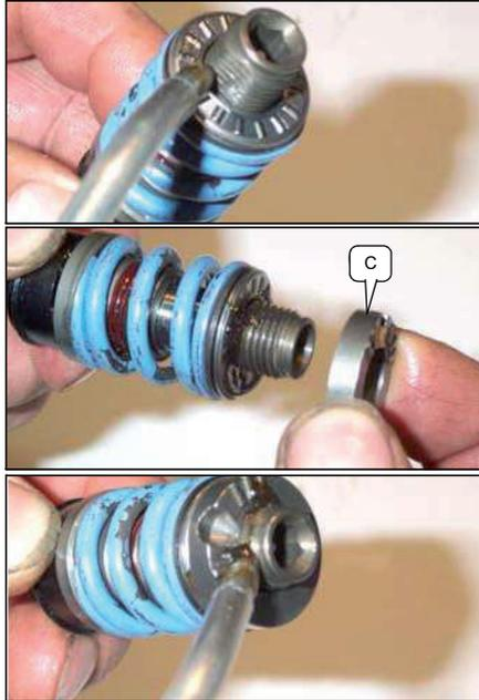
Thread on adjusting nut B.
