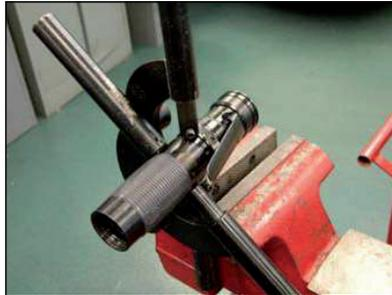
Rotate the rotor by hand to ensure it is moving freely.
