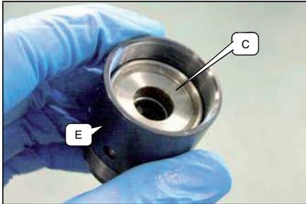
Match the teeth and slide pinion/bearing A/B into gearcase E.
