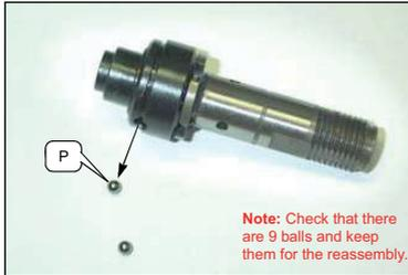
Once all ball bearings are removed, separate the clutch cam Q and the clutch driver R.
