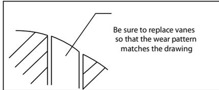
After inserting vanes into rotor, slide cylinder F over the rotor and front endplate.
