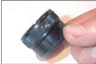
Apply grease in selector spring hole in reverse valve E and assemble spring H.
