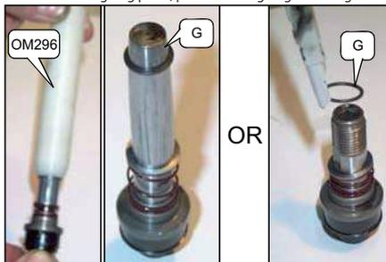
Ensure the ring is correctly positioned in the stop.
