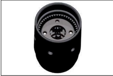
Assemble pinion adapter A into bearing B and press, supporting bearing by inner race.
