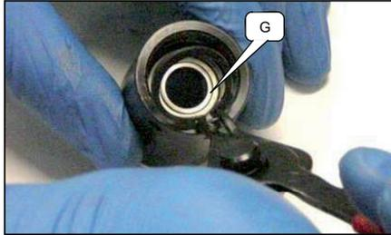
Place gearhead assembly D into gearcase E and manually press it onto bearing F. Note: support bearing by inner race.
