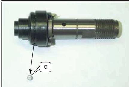
Remove the 9x3.18mm ball bearings P and save them for reassembly.
