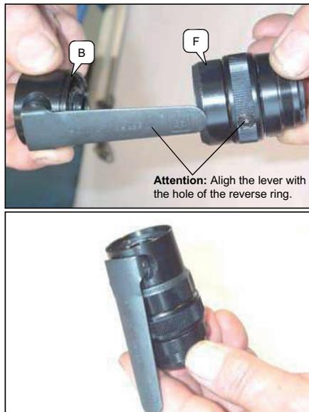
Place the ball D in the lever housing B.
