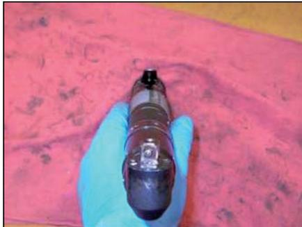
Using the spanner wrenches, tighten lock nut to 50 N-m (R25), 60 N-m (R28), 85 N-m (R35 3/8"), or 100 N-m (R35 1/2").
