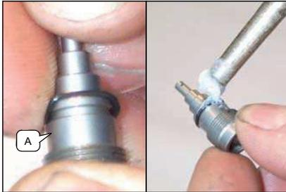
For shutoff tools, thread valve guide A into housing adapter C using a flathead screwdriver.
