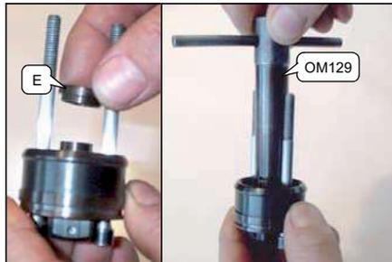
Verify that the depth of nut E has been threaded to a minimum depth of 8.5mm.
