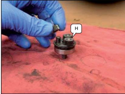
Grease the planet gears with 2cc's of IR 90 grease and slide them into the motor housing.
