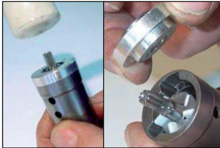
Remove old vanes from rotor and using degreaser Clean all surfaces of rotor and endplate. Oil all surfaces of the new vanes and insert them in the motor.
