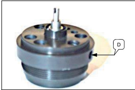
Apply o-ring lube in selector hole on housing adapter C and put ball G in place.
