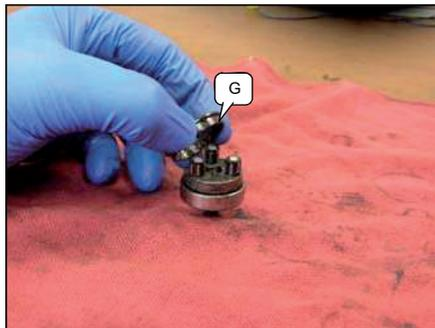
Slide planets H over the needle bearings.
