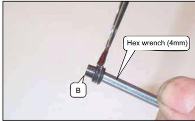
Hand tighten the screw B into reverse ring C (ring should turn freely without binding).
