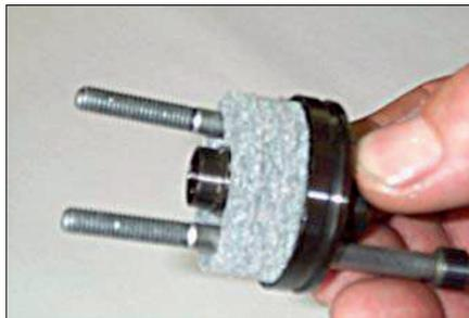
Place the diffuser C on top of the mufflers.
