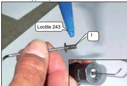
Place the motor spline into the spline adapter (previously tightened into the vice jaws) and slowly tighten screw I.
