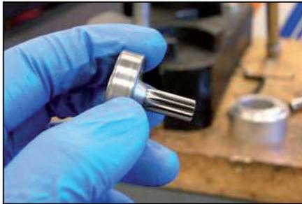
Place laminated washer into bearing cap C and assemble into gearcase E.
