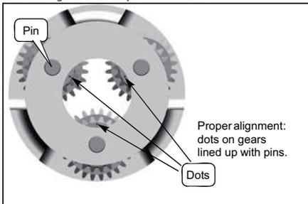
Slide gearhead assembly D and then the bearing cap C into gearcase E. Place laminated washer on bearing cap.
